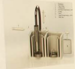
Figure 1. Diagram of the stage break sampling system.
